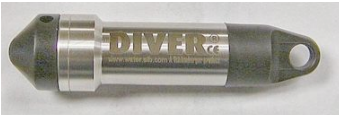
Data logger that is typical of professional data loggers used for water depth measurement
