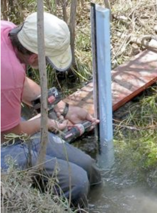
Steve Peerman installs a metal gauge on a post in the Government Spring pool formed by the installation of a weir. Later the temporary data logger installed at the Turtle Junction location in the cave was moved to the Government Spring location.
